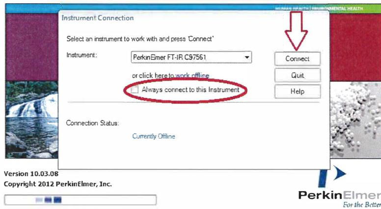
7.2.3. Make sure the Instrument being used is selected and then click “Connect”.
